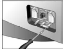
**Attention:** As loose mounting screws on the terminals could cause bad contact, make sure that they are firmly attached. However, if you overtighten, there is a risk of damaging the terminals themselves. Please use the supplied hexagonal driver and tighten screws with reasonable torque, by hand only. **Do not use powered screwdrivers of any type.**
